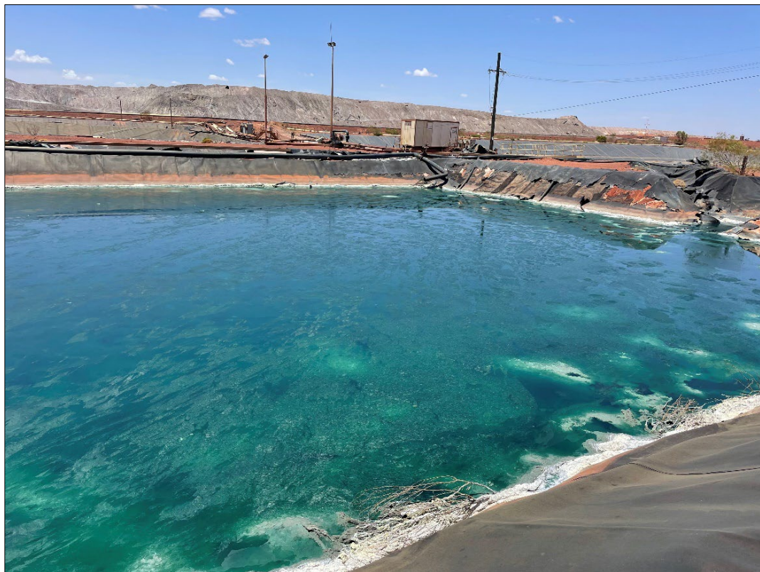
Figure 9-2: Pregnant leaching solution in pond
